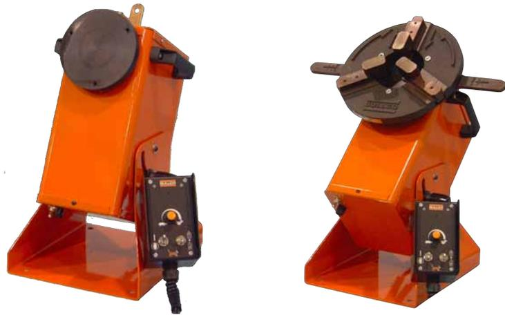
Table on the Gullco Model GP/GPP-200 Series of Welding Positioners (above left) is designed for mounting the WPG-250 Welding Gripper as indicated.
