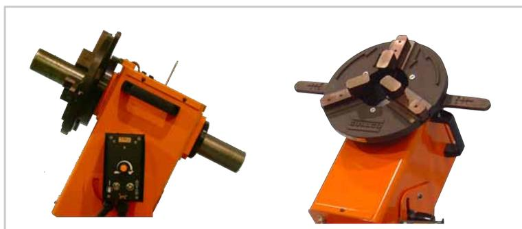
Quickly and easily mounted on any make of positioner, turntable or tailstock using three bolts provided with the gripper.
