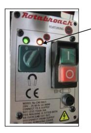
Indicator turns orange when too much pressure is added on the cutter. Will turn Red and cut power to motor if machine is given too much force for the motor to cope with.
