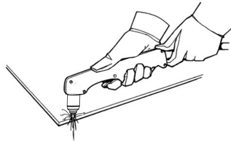
3. Drag the torch lightly across the workpiece to proceed with the cut. Maintain a steady, even pace.
