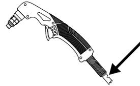
Inspect the torch lead. Replace if damaged.
