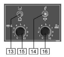
Torch Mode Switch: It enables selection of 2-step or 4-step torch mode. The functionality of 2T/4T mode is shown in the picture below:
