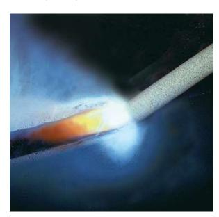
The coated electrode or welding rod serves to create the electric arc.
