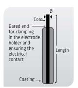
The coated electrode or welding rod consists of a metallic core centred within a coating.
