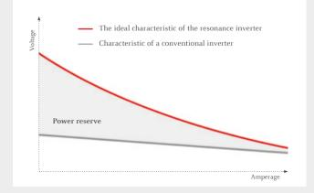
$/\,The\ resonance\ concept\ makes\ possible\ a\ near-perfect\ approximation\ to\ the\ principle\ of\ the\ ideal\ characteristic.$
