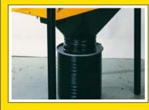
Smart"One" includes a 60° incline dust transport hopper and dust drum.
